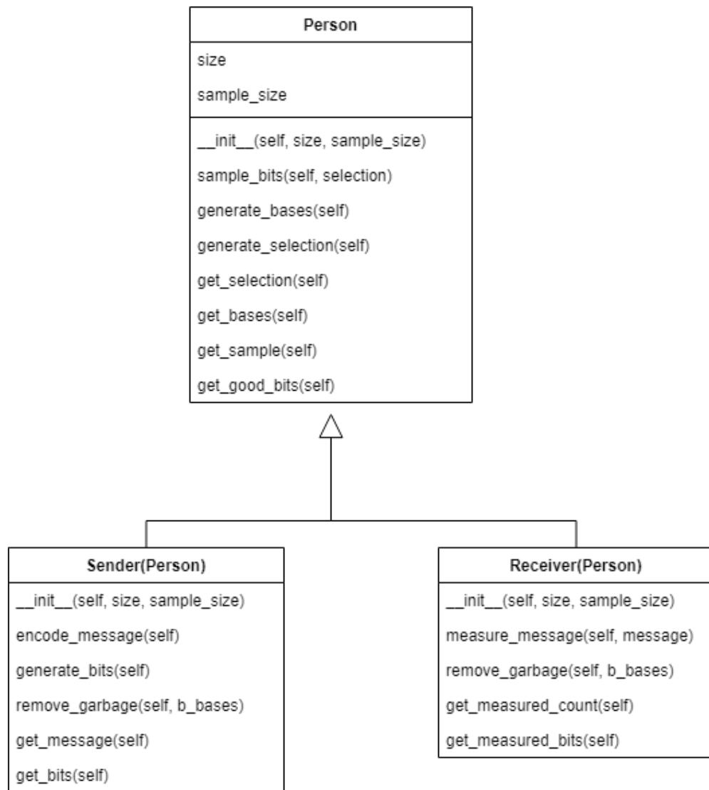
Figure 3.5 Class diagram for simulation both with and without interception
