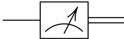
Figure 2.7 Measurement represented in a circuit 3
